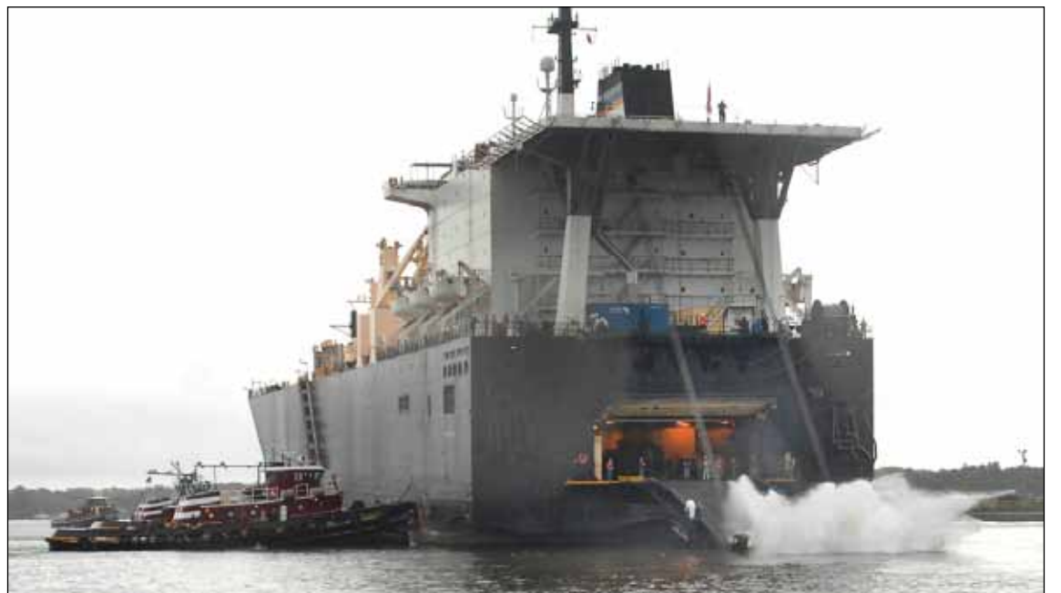
The U.S. Naval Ship Pfc. Dewayne T. Williams holds steady in Marine Corps Support Facility Blount Island's slipway adjacent to the St. John's River, as an assault amphibious vehicle launches. Nine AAVs were launched making this the first time in several years that tracks have splashed from a Maritime Prepositioning Force ship.
